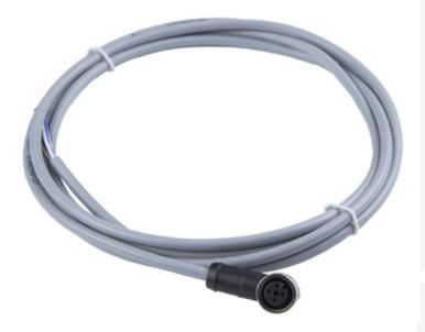
Schneider's 4-pin angled female connectors available pre-wired with cable length of 2 meters. No wiring required, can be easily connected to XMLP pressure transmitters via M12 threaded connector, resulting an IP69K rated assembly well protected from dust and water ingress.
