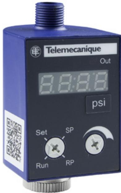
Combined with a pressure transmitter, the ZMLP switch with display converts an analogue signal into one or two switching outputs with adjustable thresholds. It can also be used to display the measured pressure. One of 27 display ranges, from -14.5 to 6000, can be selected for this purpose, meaning the switch can adapt to the majority of pressure transmitters, whether calibrated in bar, psi or pascal.
